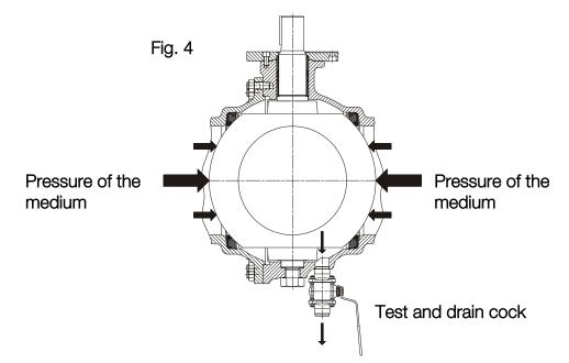
Furthermore, repair work can also be carried out on a depressurized section between the two ball valves belonging to the pressurized pipe without hazard: The medium cannot enter the repair section.
