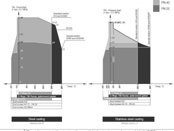
The diagrams illustrate all possible limitations of use of KLINGER valves. The area of application for standard valves is from -10 °C up to +200 °C. CAUTION Special designs with a suitable sealing system exist for the temperature range from -45 °C to -10 °C as well as from 200 °C to 260 °C.
