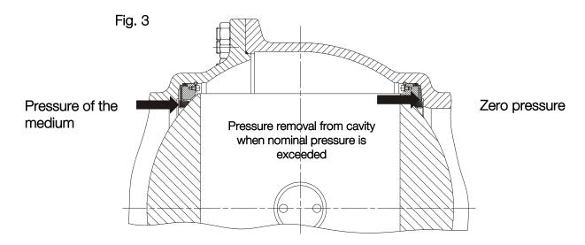
The ball valve can be pressurized in both flow directions. Thermal expansions are compensated by the elasticity of the sealing elements.
